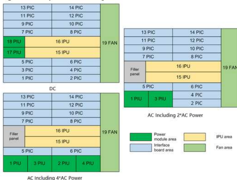
Figure 7 Slot Layout of the NetEngine 8000 M14
